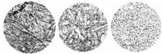
Martensite, tempered martensite and heavily tempered martensite
