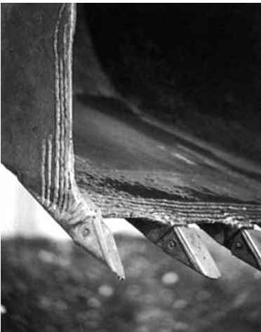
Overlay. Bucket lip hard surfaced as preventive maintenance
