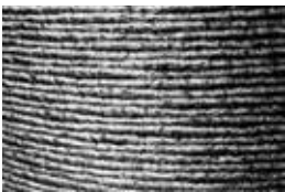
Stress relief cracks in a high chrome carbide overlay
